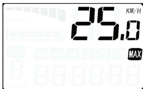
★ Press UP or DOWN to enter into speed-limit value selection. Reference speed limit values 20~40KM/H.
